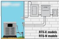
Use service rated (D, J, CSA models) with service disconnect for quick & easy installations. Use non-service rated (X, N models) for custom installations or with installs that require a subpanel.
